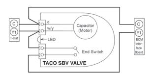
Fig. 33 — Taco SBV Valve Wiring
